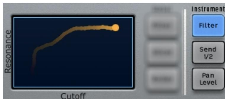
The Filter type for the kit is determined by the setting for the Global Filter button, but SparkLE allows you to apply this effect to one instrument at a time rather than the entire kit, if you like. To do this, select an instrument such as the snare (press Select + Instrument pad 2), then press the Instrument Filter button (pictured). Now the Live FX pad will alter the filter frequency and resonance for the snare only.
