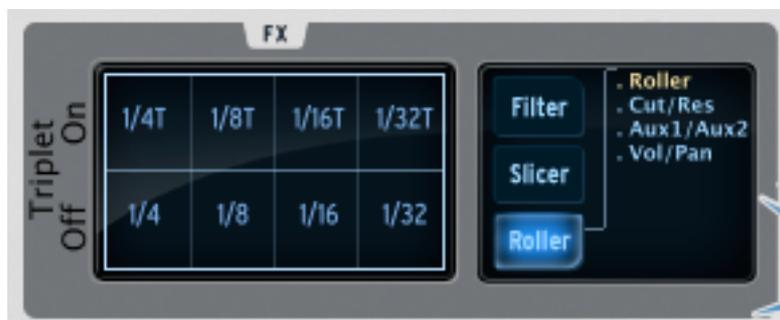
Choose the note value for the Roller effect. Then, click and maintain your click on the snare drum pad. The snare drum will play a basic drum roll. The roll speed depends on the selected note value.
