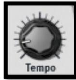
The Tempo knob allows you to set the tempo for your pattern when SPARK is not externally synced to a host. The internal Tempo range is 10BPM to 300BPM.
