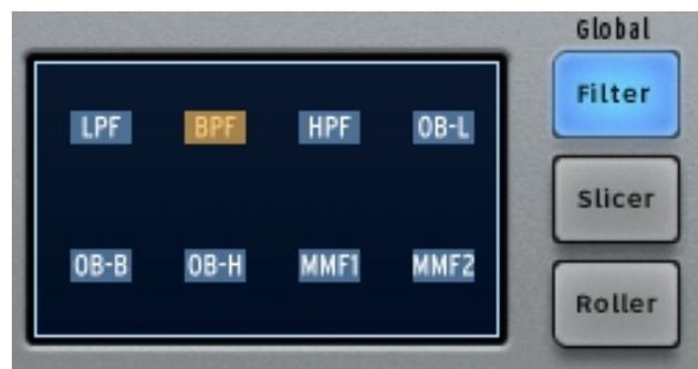
The Filter button offers proprietary Low pass, Band pass and High pass filters, plus Oberheim-style Low, High, Band pass and Multi-mode filters, each with cutoff and resonance.
