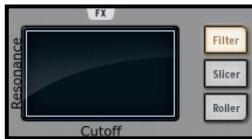
The FX Live pad is an amazing performance tool, especially if you plan on playing live. Its touch sensitive screen will apply live effects in real time to your song or patterns, allowing you to shape your sound with great precision. When your cursor enters the FX pad zone, it turns from an arrow to a cross.
