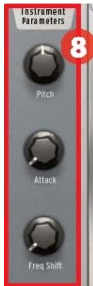
The three knobs on the right side of the Center panel control the selected instrument's parameters. Let's say you want to change the pitch of the bass drum, for example. First click "Select" and then click the bass drum pad. After this the Instrument Parameter knobs will show which three parameters have been selected for the bass drum: in this case, Pitch, Attack and Freq Shift.
