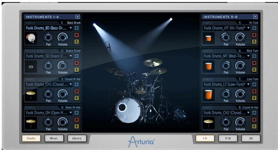
The studio panel displays all your instruments as well as their parameters. From here you can load instruments into slots, apply filters and effects, etc. The picture above shows the 1-8 instrument view. Let's look at the Bass drum window:
