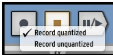
In Quantize mode; the recorded notes will be set exactly to the nearest step position. When quantize mode is disabled, the recorded notes will keep the exact position they were played on. Spark uses the Shift parameter (see section 6.5.5 to remember the exact triggering time relative to a step position.
