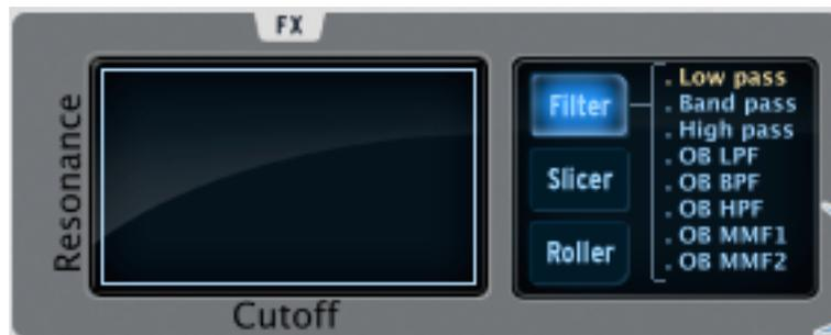
The Filter button offers a Low pass, a Band pass and a High pass filter, Oberheim Low, High, Band and Multi-mode filters with cutoff and resonance.
