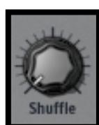
This knob sets the amount of shuffle applied to a pattern. Shuffle is a rhythmic shifting of a Pattern in which the first note in a series of two plays for a longer time than the one that follows.
