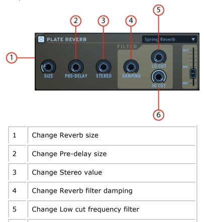
A reverb emulates the reflections of a sound in a different space (room, hall, etc). Reverb adds depth and richness to a sound by 'placing' it in a separate physical space. The size knob changes the size of the space. Predelay adds a small amount of delay to the sound to imitate early reflections. Stereo refers to the width of the stereo field of the reverb. Dampening sets how much the reverb should be filtered using the Lo and Hi Cut filter settings.
