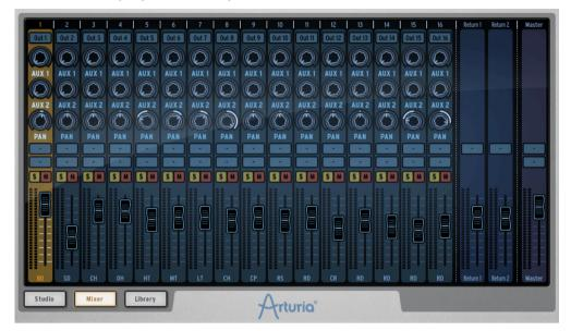
This panel is your 16 channel mixer panel. This is where all your instruments will be mixed together. Here, the modified signals will be summed to produce the combined output signals.
