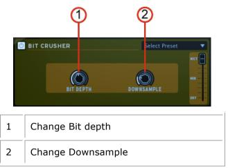
A bit crusher reduces the bit depth and sample rate of the audio signal. The result is a very digital sounding distortion.
