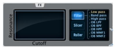
The Filter button offers a Low pass, a Band pass and a High pass filter, Oberheim Low, High, Band and MiniMoog filters with cutoff and resonance.
