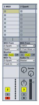
Press Record button in Live. Note that Host and Tempo button must be on in Spark software.
