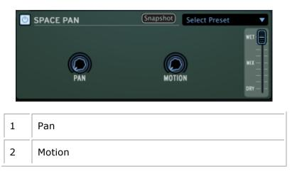
Space panning is the spread of a sound signal into a new 3D sound field. The sound will be set at a position or automatically (Pan set to 0) and the position will be modulated with the motion parameter. Space pan must be used on stereo sounds.
