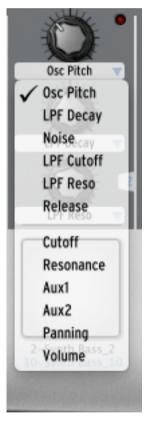
Click on a different parameter name to assign the knob to that parameter. To select different parameters via the hardware controller, Press and hold SELECT and turn the knob that you want to change assignment on. You will see the different parameters in the LCD screen and on the software screen.
