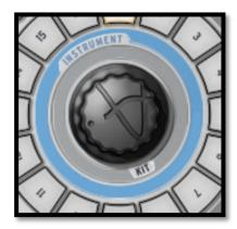
The Jog Dial allows you to load Kits, Instruments or projects when working on an open project. You may choose (via the preferences tab in the upper screen) to assign the Jog dial to switch between either Instruments and Kits using the "Switch from Instrument to Kit Mode", or else between Instruments and Projects using the "Switch from Instruments to Projects Mode". By default Spark is set to "Switch from Instrument to Kit Mode".
