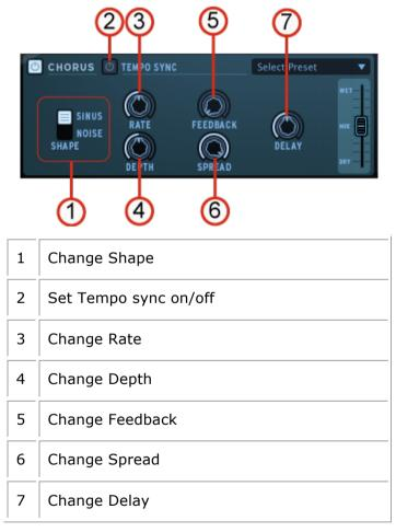
Chorus is a classic effect that uses small delay times (that are modulated by an LFO) to double a sound, making it seem fatter and thicker. Shape, rate and depth refer to the LFO. Delay is the delay time and feedback is the amount of delayed signal added back to the dry signal. Both of these parameters emphasize the effect when increased. Spread refers to the width of the sound in the stereo field.
