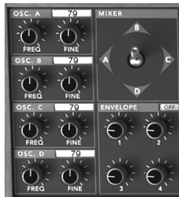
The Prophet VS oscillators and the mixing joystick
