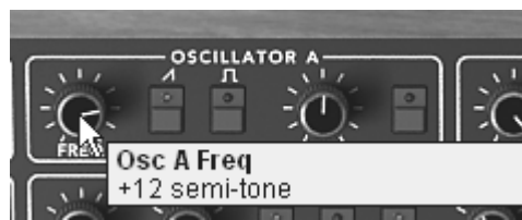
Setting the Range of the oscillator ("Frequency")
