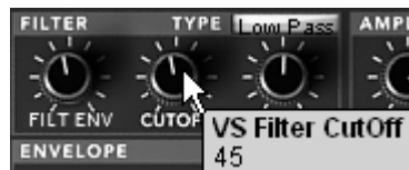
Lower the value of the filter's cutoff frequency to 45
