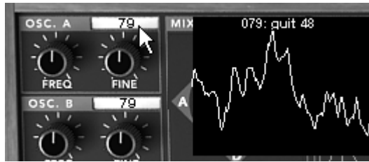
Screen for choosing the waveforms of the oscillators
