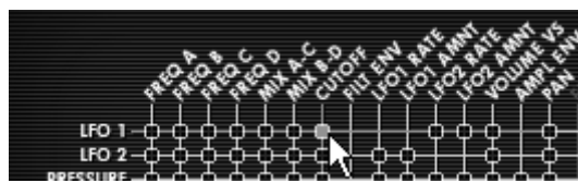
Click on the white points to add a modulation connection
