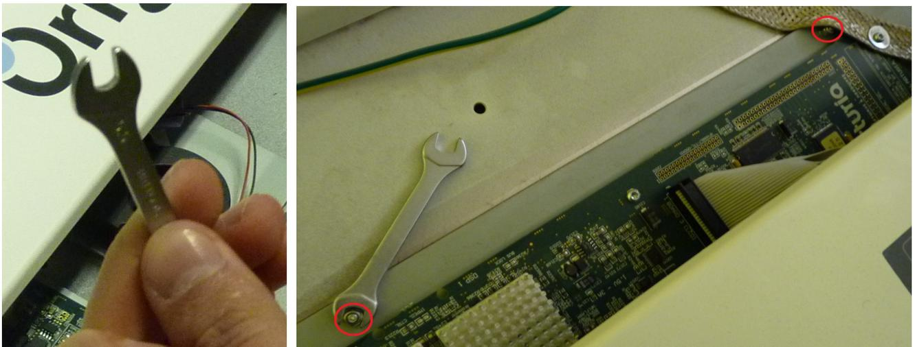
2/ Unscrew the 3 screws that retain the rear card on the metal plate by raising the unit.
