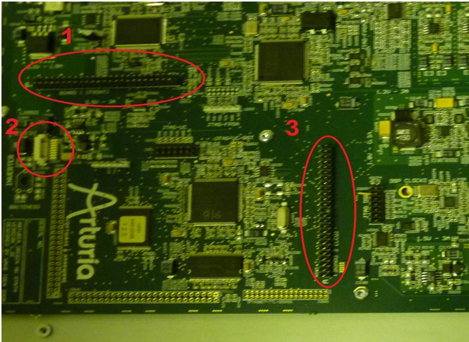
b. Remove the card by pulling the metal plate
