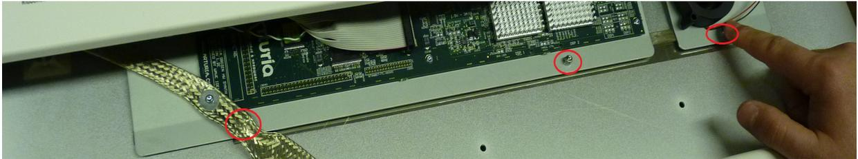
1/ On the other side use a 5:5 key to retain the nut when unscrew.
