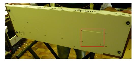
2/ Use a screwdriver to remove the four screws
