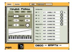
A new keyboard-follow mode has been added (mode II). It is a useful new source of modulation that can be used to emulate the CS80 keyboard follow modes.
