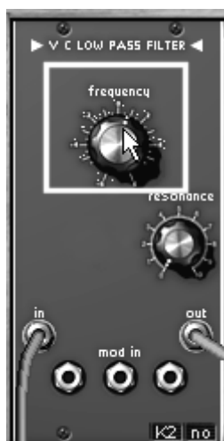
The setting of filter1 cut-off frequency
