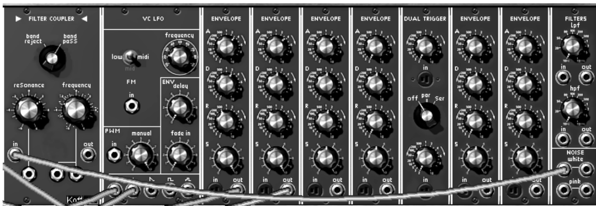
The white noise module connected to the band pass filter
