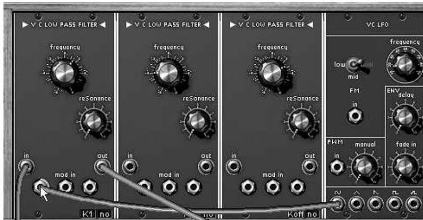
Connection of LFO to filter1
