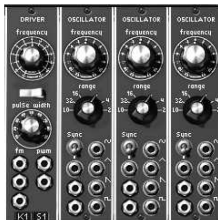
An oscillator bank: 1 "driver" and 3 "slave oscillators"
