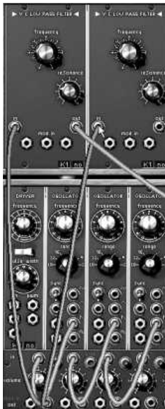
Connection towards the second filter
