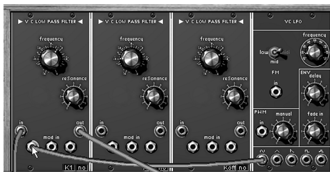
Connection of LFO to filter 1
