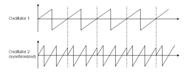
In the image above, oscillator2 is synchronized with the first, and then tuned to a frequency with double the tonality.
