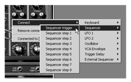
Apply a sequencer output to the VCA (here VCA2)
