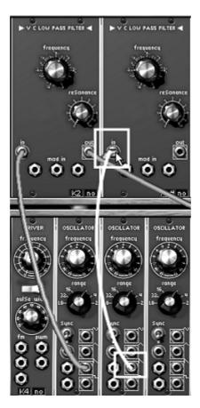
Connection between oscillator 2 and filter2
