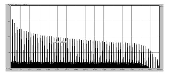
Linear frequency spectrum of the Moog Modular V oscillator made with TAE®
