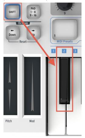
Then when it's time to switch to channel 1, for example, use the same technique but press a different key: in that case, you would hold the Shift button and press the first C key on the keyboard.
