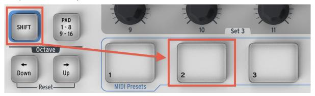
In the picture above the combination of the Shift button and Pad 2 will select Preset #2 from the MiniLab preset memory locations.
