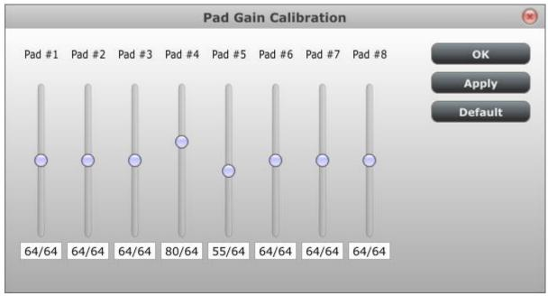
Here you can alter the pad velocity gain. Each of the 8 hardware pads has a dedicated setting.
