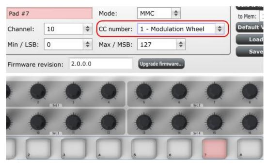
Next, select Pad 8 so we can set it to the MMC command for "Start". This means the CC number must be set to 2:
