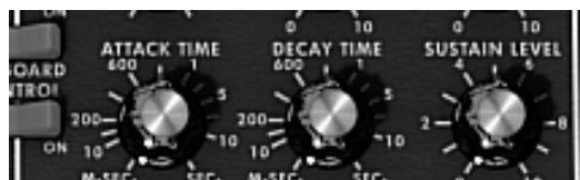
Envelope generator associated to the filter
