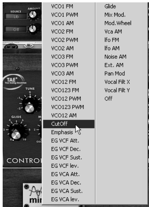
Modulation of the filter cutoff frequency by the LFO
