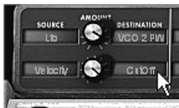
The velocity set to modulate the "Cutoff"
