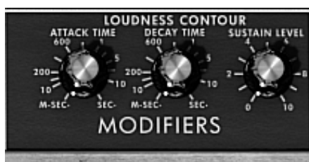
Parameters of the envelope generator associated to the VCA
