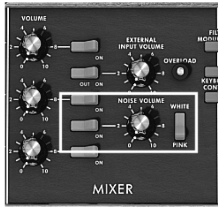
The noise generator set on the mixer
