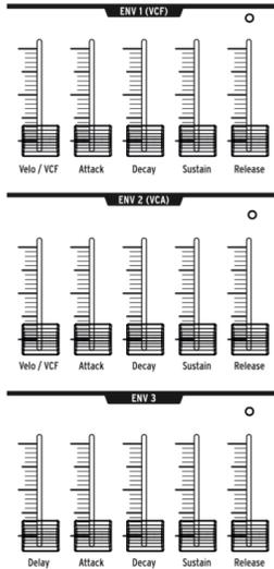
Envelopes are adjustable modulators that shape the voltage over time. MatrixBrute has two 4-stage, ADSR (Attack Decay Sustain Release) envelopes, plus a third one (ENV 3) which adds a Delay phase before the ADSR (this is all explained below). Each envelope has a "gate" LED that show when a gate is receive and will fade out to show when the release stage is still active.
