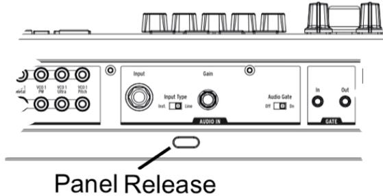
With the MatrixBrute on a solid playing surface, push the **Panel Release** latch and use the hinged prop inside to set the control panel at the most convenient angle (or just leave it flat if that works better). Take care when lifting on the Matrixbrute panel as it could cause the support to fall.
