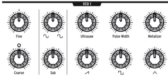
The only difference between these two VCOs is that VCO 1 can be routed into VCO 2 to modulate it (this is called *frequency modulation*, or FM). Both VCOs operate the same way.
