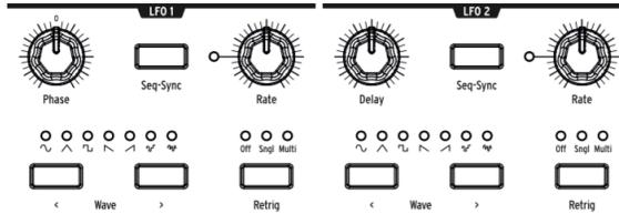
The two LFOs (low frequency oscillators) are modulators that can be routed to add movement to pretty much any parameter on the MatrixBrute. LFO waveforms are near or below the bottom threshold of our hearing, ranging from about one cycle every 18 seconds up to 100Hz. They're useful for creating all kinds of sounds, from vibrato to filter sweeps to pitch changes; their effects range from subtle to wild.
