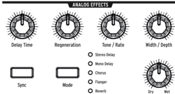
MatrixBrite features Analog Effects with 5 different modes on the output.
