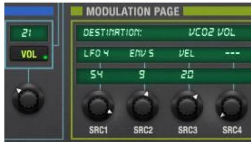
Note the small green LED in the lower right corner of the VCO2 VOL button, pictured above. Even if a mod is not in focus on the Modulation Page, an LED like that will remain lit inside the mod button of a parameter when it has an active modulation routing.
