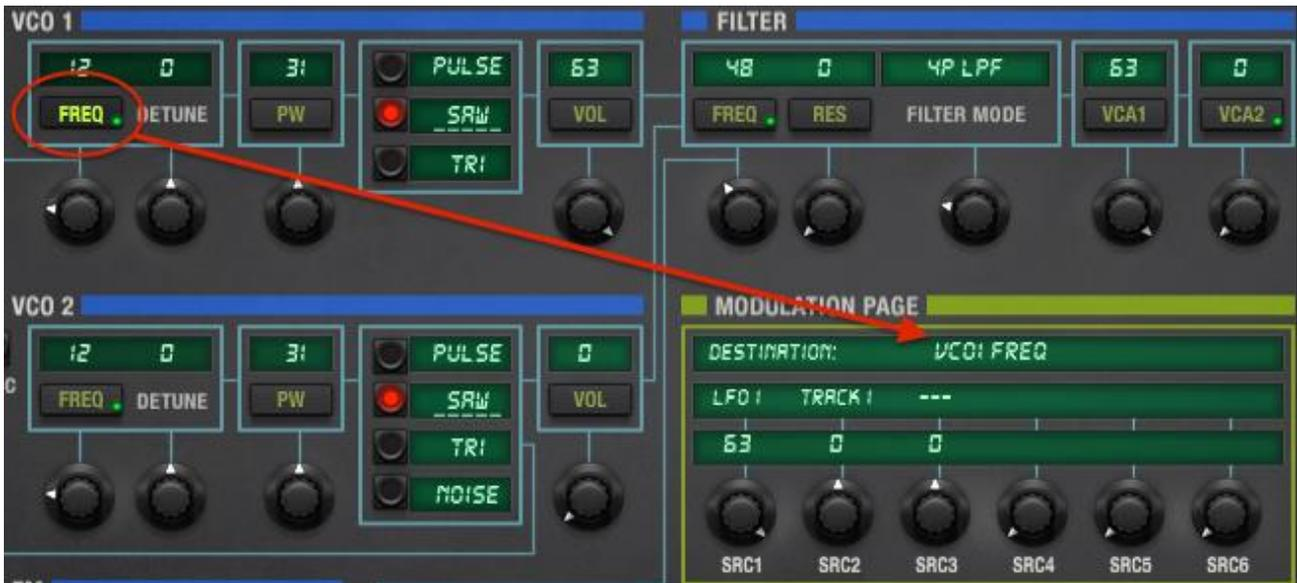
In the above picture the VCO 1 Frequency mod button has been selected, bringing that parameter into focus in the Modulation Page. We can see that both LFO 1 and Tracking Generator 1 are selected as modulation sources, although the mod level for the Track 1 mod is set to 0 so it is having no impact on VCO 1.
