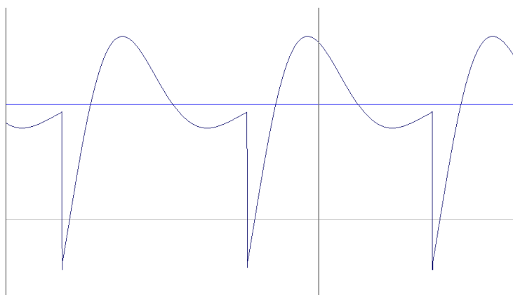
Temporal representation of a sawtooth waveform, deformed by high-pass and low-pass filtering, of the original CS-80
