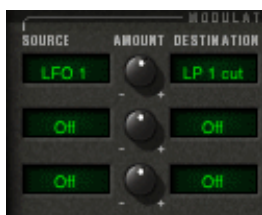
Modulate the frequency of the low-pass filter (LP 1 cut) with the LFO (LFO 1)
