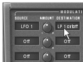
Modulate the frequency of the low-pass filter (LPF1) with the LFO (Sub 1)
