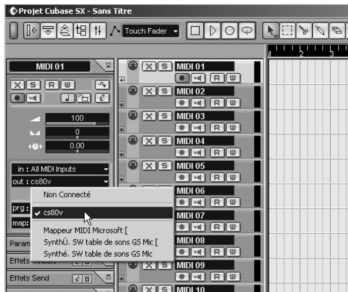
Connection of a MIDI track to the CS-80V
