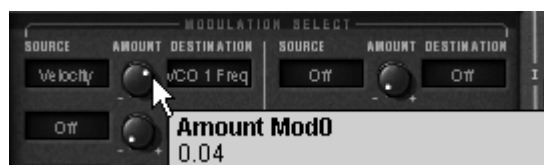
Apply the velocity on the frequency of oscillator1
