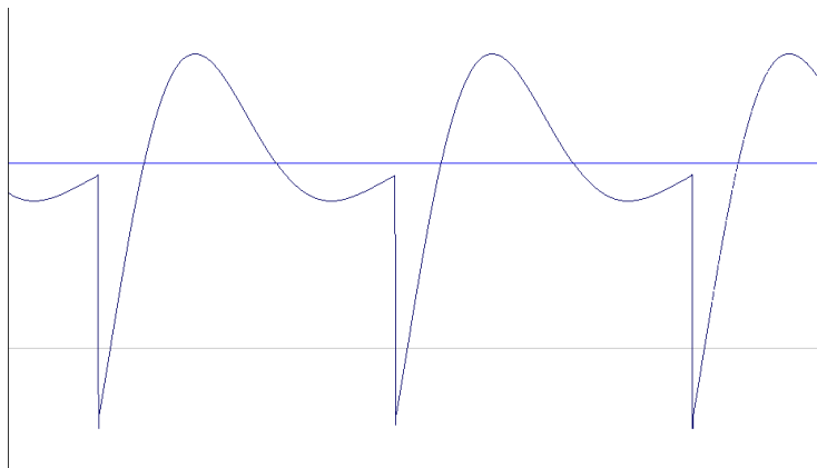
Temporal representation of a «saw tooth» waveform (deformed by high-pass and low-pass filtering) reproduced by TAE
