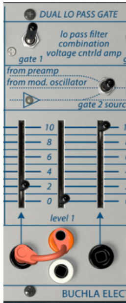
The Dual Low Pass Gate as a filter
