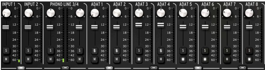
When the Digital Input is set to ADAT and one of the two lowest sample rates is selected, 8 ADAT channels will be shown.
