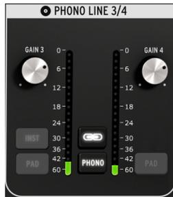
When the Link button is clicked the Gain knobs will jump to the lowest of their two values. After that, when one knob is turned the other will turn also.
