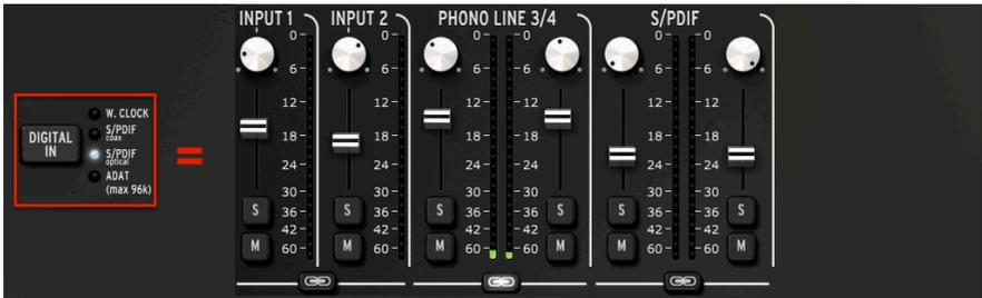
Another pair of audio channels are added when the Digital Input is set to one of the two S/PDIF inputs (coaxial or optical). All sample rates between 44100 and 192000 are available.
