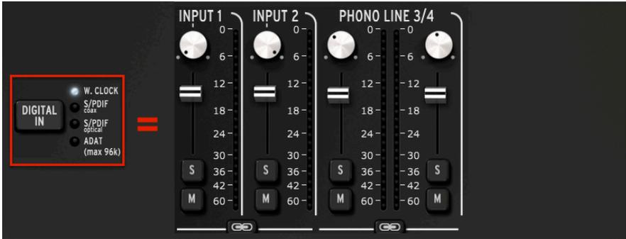
This is what you will see for all sample rates when Word Clock is selected for the Digital Input. It is the most basic configuration, with only four audio channels in use.
