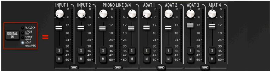
The maximum sample rates for an ADAT input are 88200 and 96000. At these rates only four channels of audio are being transmitted by the ADAT device to the AudioFuse, and so only four channels are displayed in the Direct Monitoring Mix window.
